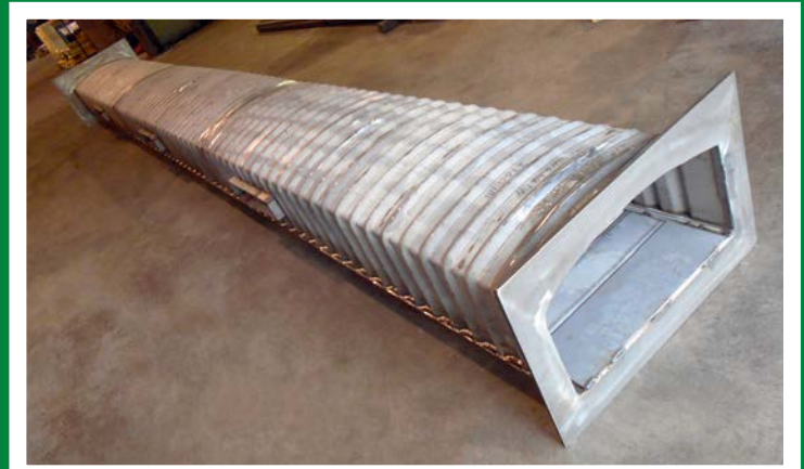
Corrugated Muffle with Stainless Steel Hearth Plates
