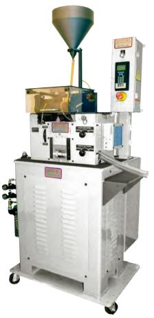
Anvil pressing is a 'natural' for parts with one flat side. The other side can be flat or multi-level. The parts can have holes, teeth, etc. Our patented Unitized Anvil design combines the powder feeder, anvil and vacuum pick up into one unit which is always in contact with the die plate., virtually elimination powder spillage. Parts are compacted against an anvil by the upward action of a lower punch. There are no upper punches and associated problems of misalignment, breakage and wear.
