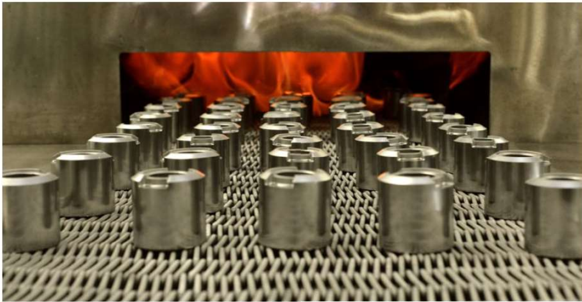
Fig. 10 PM parts entering a mesh belt sintering furnace
