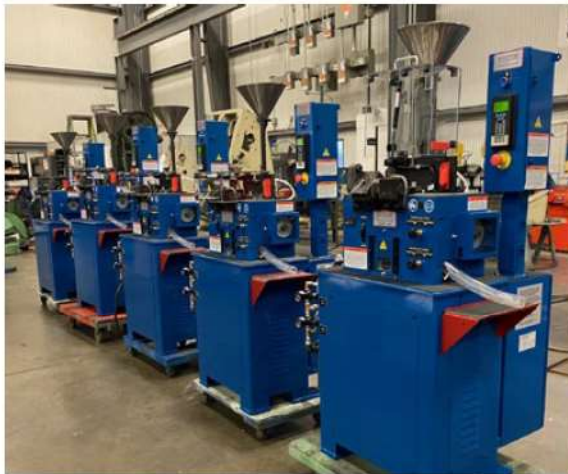
Fig. 6 A group of five Pentronix high-speed mechanical presses in DuBois press assembly and test shop
