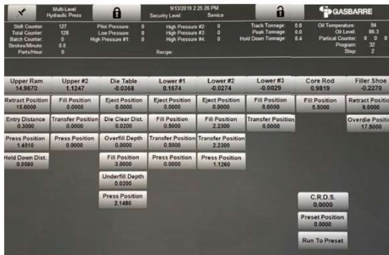
Fig. 8 HMI (Human Machine Interface) on a dry bag isostatic press
