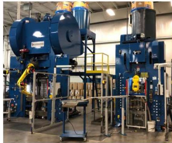
Fig. 7 Mechanical presses with robotic automation in production
